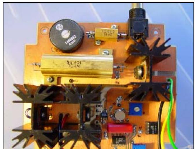
Fig. 4. The prototype model of, the Buck converter with the sliding mode control build in the Electronics laboratory at Lappeenranta University of Technology.
