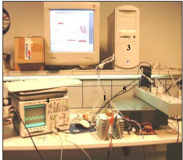
Fig.4. Test set-up consisting of the: Buck-Boost converter (1), connector panel (2), host pc with dSPACE™ DS1103 card (3), oscilloscope (4), and input voltage source (5).
