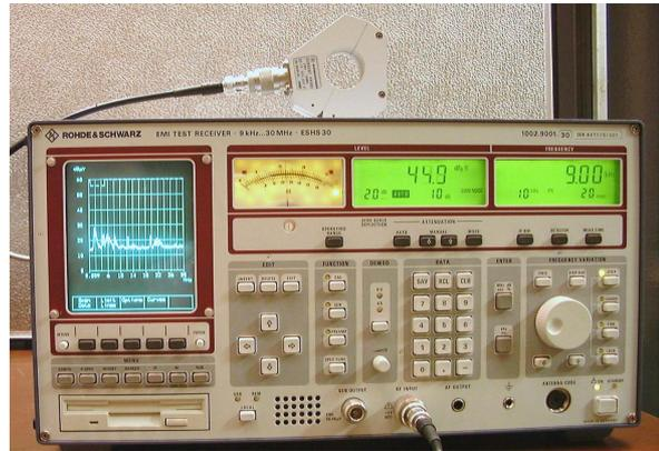
Fig. 12: Rohde&Schwarz EMI test receiver and the current clamp used in the measurements.
