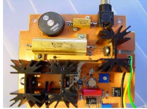
Fig. 1. Simplified prototype circuits of the HWZCS DC/DC converter with PI and current hysteresis control, the combined loops perform SMC. A gate drive circuit is used to provide isolation to the switch.
