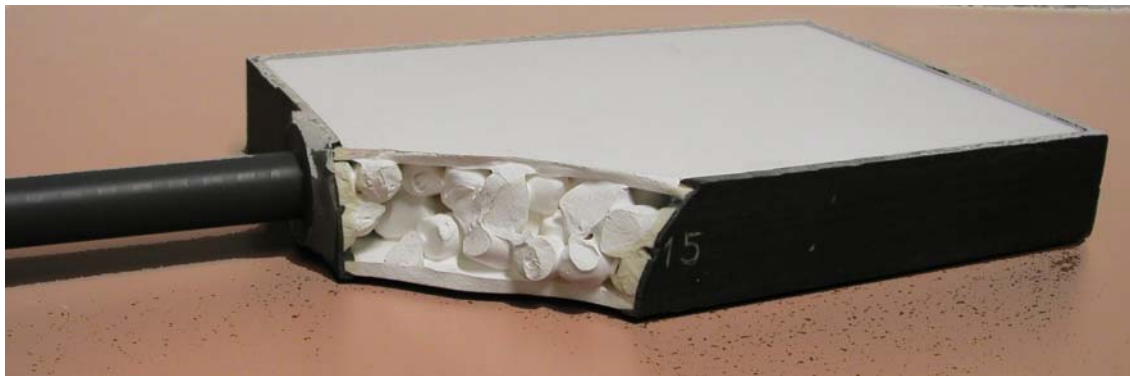
Figure 6 A photograph of the type of ceramic membrane used.
