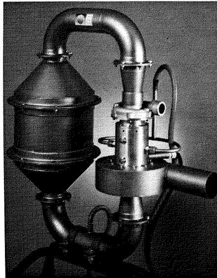
Figure 35. Test Facility II, sub-pressure connection. The rotating part vertically in front in the order: compressor, motor and turbine. The droplet separator can be seen at the back. Photo vesa Mikkonen
