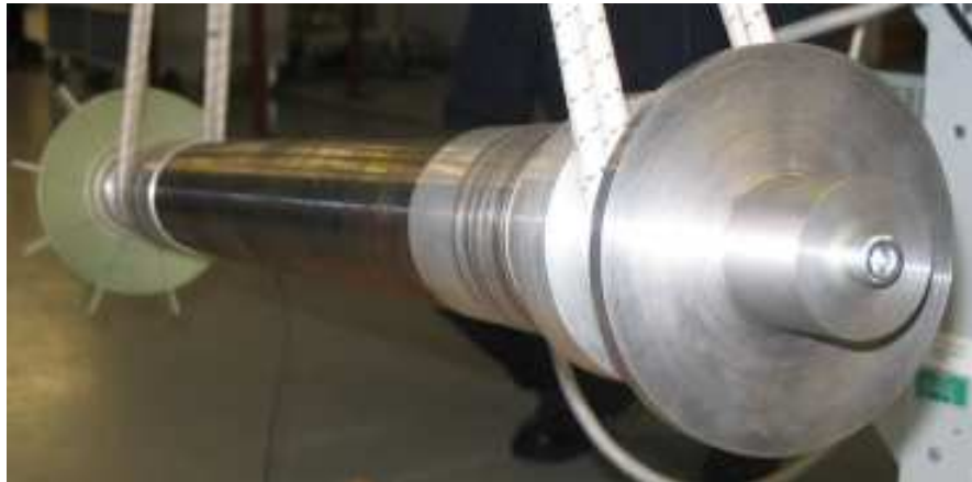
Figure 3.7: Complete rotor, under the modal analysis, consists of the shaft, axial disk, propeller coupling, AMB laminations fitted with aluminum sleeves, and additional aluminum sleeves for the position measurements.
