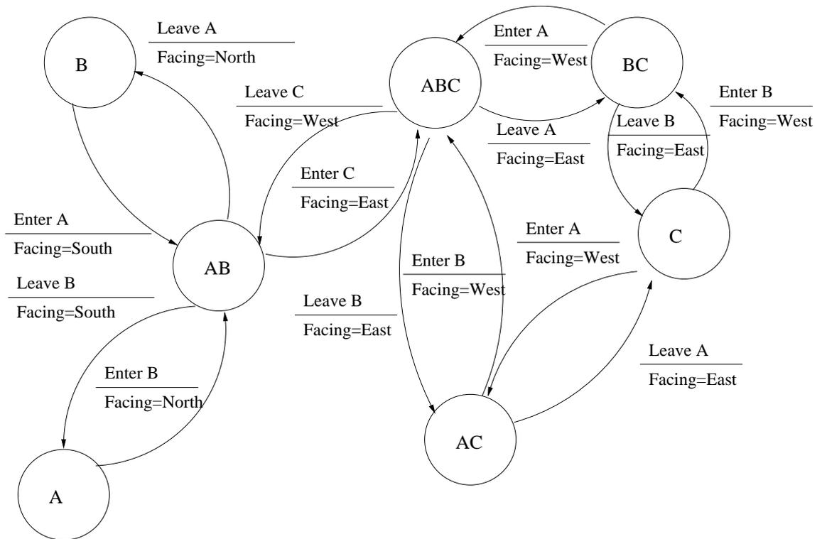
Figure 12: Statemachine for the user movement in figure 11 covering guides A,B and C
