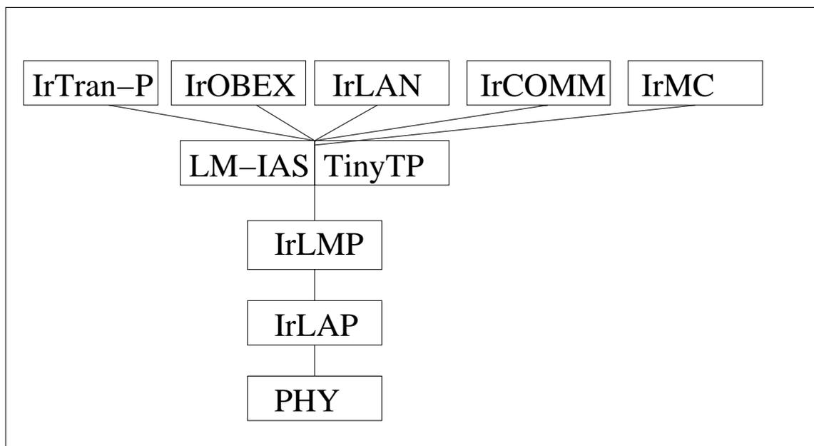
Figure 2: IrDA data protocol stack
