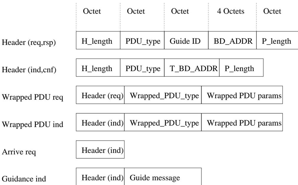
Figure 8: PDU's between guide and server
