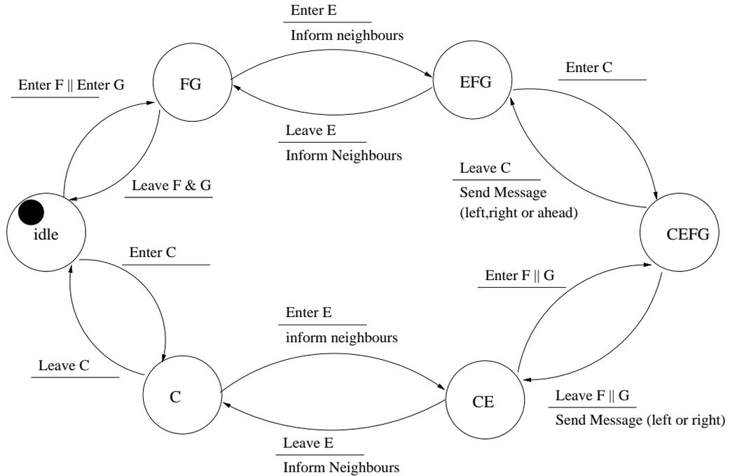
Figure 14: Statemachine for guide E in figure 13
