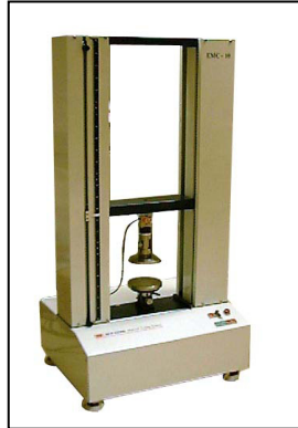
Figure 8. Edgeboard testing machine (Eltete Sales and Marketing meeting CD-Rom 2003)
