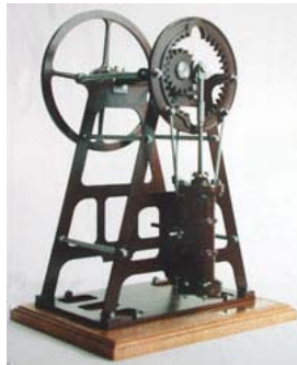
Figure 2.1.1. Murray's hypocycloidal steam engine [Clarke 2006].
