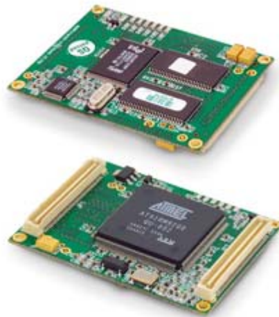
Figure 2. Selected Processor Module, Garz & Fricke ECO920 (Garz & Fricke 2008).
