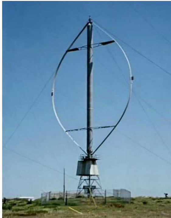
Figure 4.3. Darrieus Vertical-Axis Wind Turbine. (DVAWT) (Energy, 2009)
