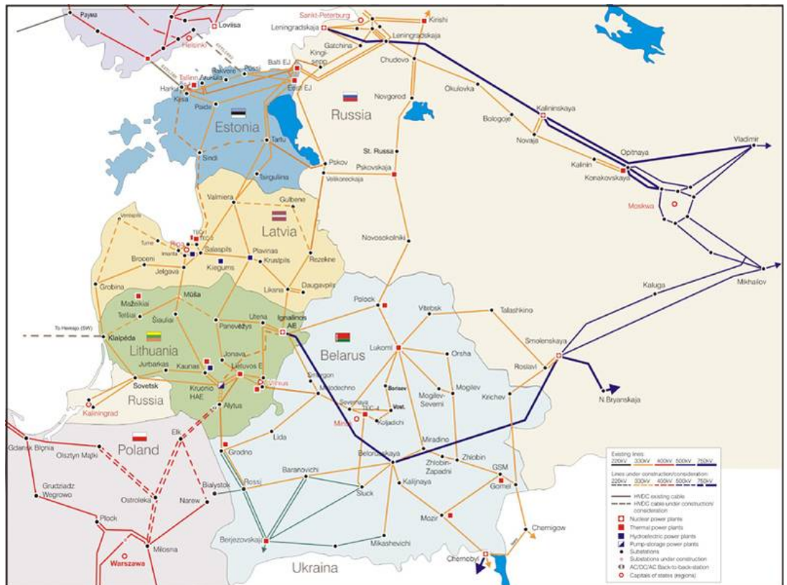
Figure 1. Electrical Ring of the BRELL network 330-750 kV (Armis Staltmanis 2006)
