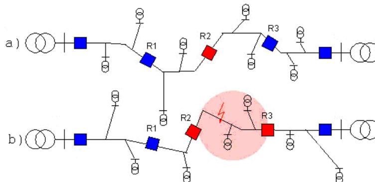
Figure 7. Decentralized automation of distribution feeder a) network state before the fault, b) network state after the fault, R1, R2, R3 – reclosers, area de-energized after the fault is shown in red circle (Vorotnitsky)
