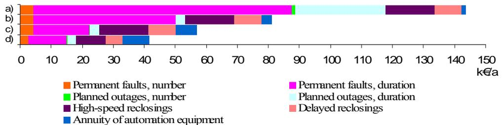
Figure 33. Costs structure of case feeder when a) no switching equipment installed; b) 9 MCDs installed; c) 5 MCDs and 4 RCDs installed; d) 5 MCDs and 5 reclosers installed
