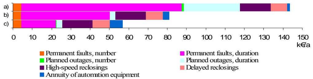
Figure 29. Costs structure of case feeder when a) switching equipment installed; b) 9 MCDs installed; c) 5 MCDs and 4 RCDs are installed.
