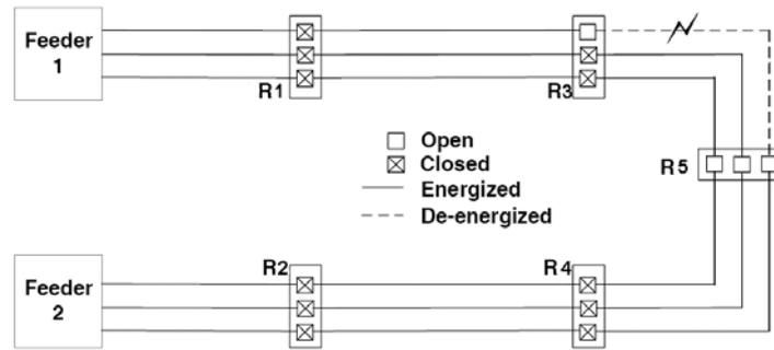
Figure 9. 5-recloser loop scheme (Taylor et al. 2008)
