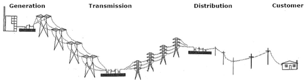
Figure 1. Transmission and distribution of electric energy
