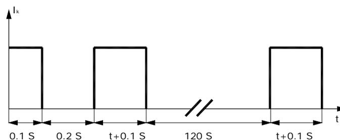
Figure 14. Autoreclosing cycle in permanent fault
