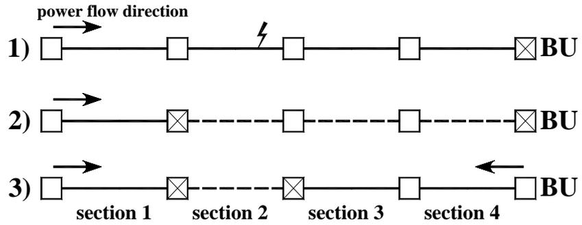
Figure 21. Sequence of switch states during the fault at feeder section 2
