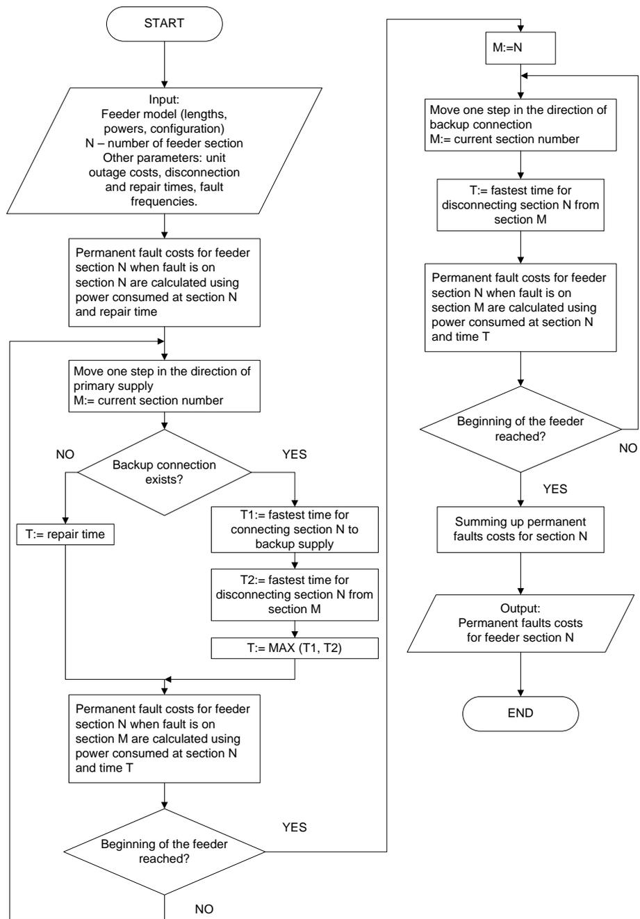
Figure 19. Flowchart for calculating permanent faults costs
