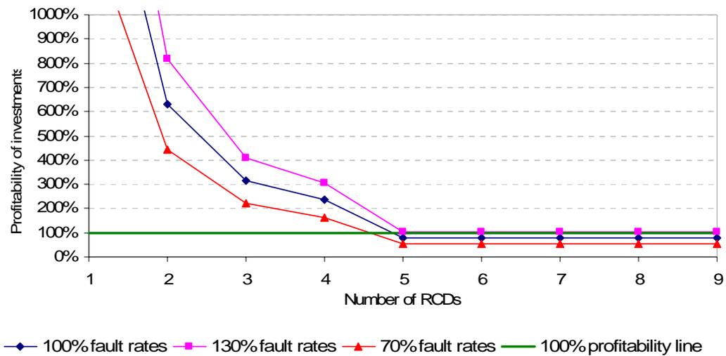
Figure 36. Dependence of RCDs profitability on variation of fault frequencies. 100 % corresponds to values given in Paragraph 4.1.5
