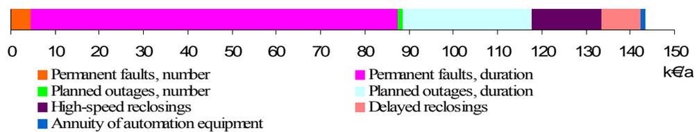
Figure 22. Costs structure for feeder with no automation installed
