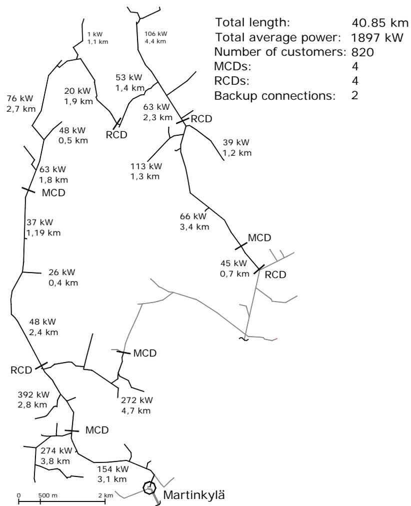
Figure 37. Case feeder. MCD stands for manual controlled disconnector and RCD for remote controlled disconnector.
