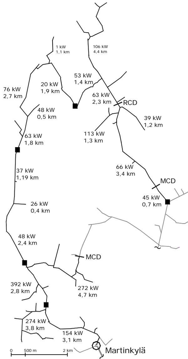
Figure 50. Feeder structure after renovation with five new reclosers.
