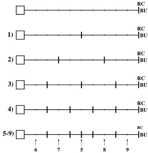
Figure 23. Order of manually controlled disconnectors installation
