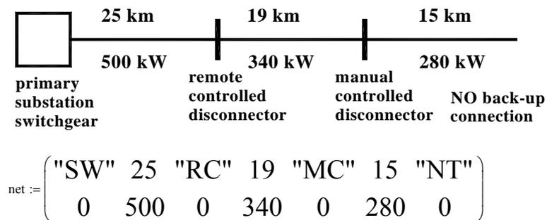
Figure 20. Example of feeder configuration and its matrix representation for reliability model
