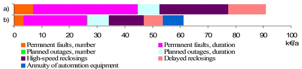
Figure 45. Costs structure a) before renovation; b) after 5<sup>th</sup> step of renovation
