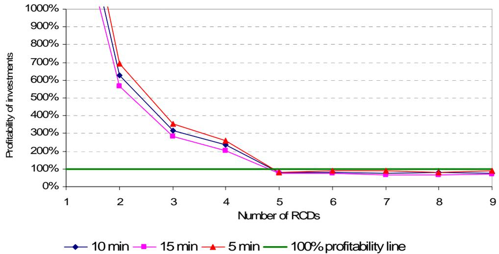
Figure 34. Dependence of RCDs profitability on variation of RCD disconnection time.
