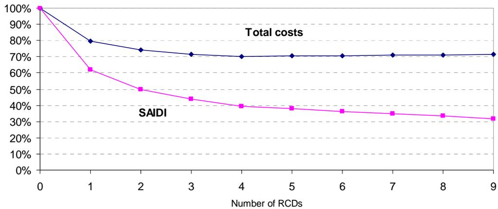
Figure 27. Influence of RCDs on SAIDI and total costs. Level of 100 % illustrates situation before automation installation.
