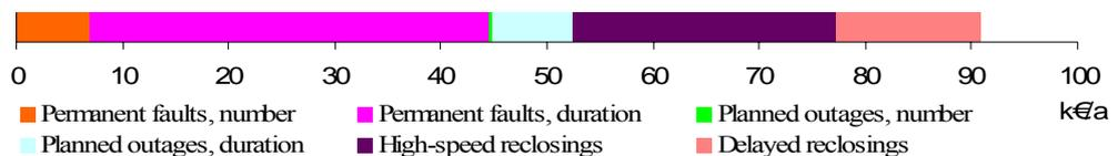
Figure 41. Outage costs of the case feeder before renovation.
