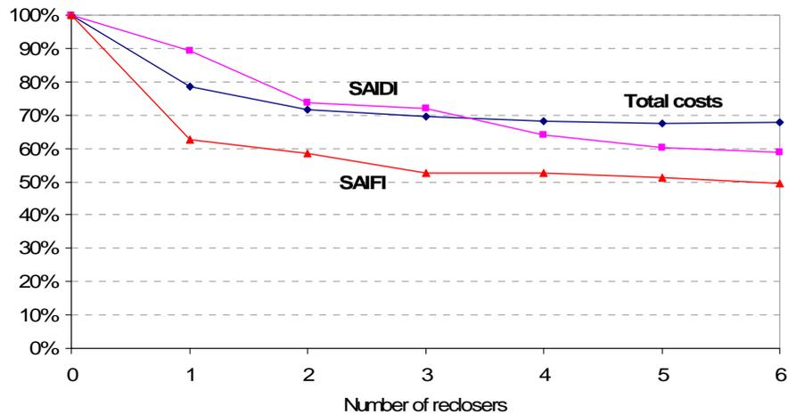
Figure 43. Results of step-by-step renovation
