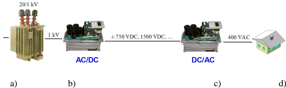
Fig. 1.1. A simplified structure of a low-voltage DC delivery system. a) distribution transformer, b) AC/DC rectifier, c) DC/AC inverter, d) customer. The converters (b and c) may be two or four quadrant converters depending on the need of power flow direction. If there is no generation in the distribution system the AC/DC converter (b) may be a two quadrant converter. If there is generation the AC/DC converter (b) has also to be a four quadrant converter as the customer DC/AC converter (c). (Lassila 2008)
