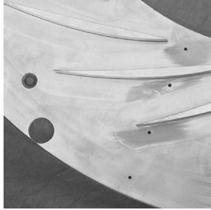
Figure 5.4: Details of the static pressure taps in the diffuser and cobra probe traverse location after the diffuser.
