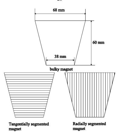
Fig. 1.5. Magnet versions, slicing directions.
