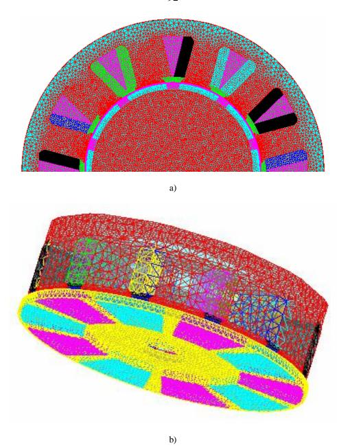
Fig. 4.3. Mesh figures in a) radial flux machine 2D FEA and b) axial flux machine 3D FEA.
