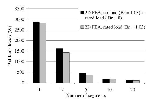
Fig. 2.14. Permeance-harmonic-caused (no load,  $B_{\rm r}=1.03$ ) and winding-harmonic-caused (rated load,  $B_{\rm r}=0$ ) PM Joule losses calculated by the 2D FEA compared with the total harmonic-caused (rated load,  $B_{\rm r}=1.03$ ) PM Joule losses calculated by the 2D FEA for a 12-slot-10-pole- machine. One magnet is segmented into 20 pieces at maximum.
