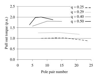
Fig. 3.3. Pull-out torques of concentrated winding machines with  $q=0.25,\,0.29,\,0.4$  and 0.5 (Jussila et al. 2007).
