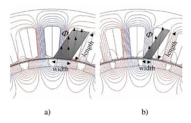
Fig. 3.8. 36-slot-24-pole motor, which has a) semi-closed slot openings with the relative slot opening width of 0.09 of the slot pitch and b) open slots with relative slot opening width of 0.6 of the slot pitch (Lindh et al. "Concentrated Wound PM Motors with Semiclosed Slots and with Open Slots." *IEEE Energy Conversion* (forthcoming)).
