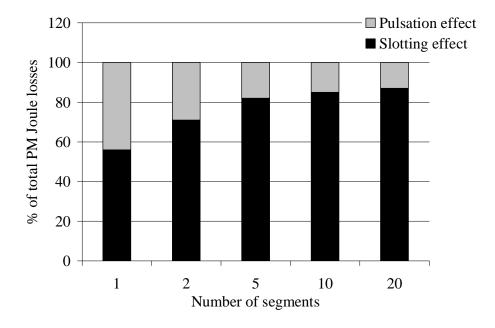
Fig. 2.20. Proportions of PM Joule losses caused by the winding and permeance harmonics calculated by the 2D FEA for a 12-slot-10-pole machine.
