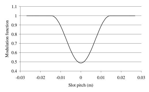
Fig. 2.18. Modulation function according to Zhu and Howe (1993) and the corresponding Fourier-series-based factors for the prototype machine are  $K_0 = 0.8618$ ,  $K_1 = -0.2282$ ,  $K_2 = -0.1219$ ,  $K_3 = -0.0312$ ,  $K_4 = 0.0052$ ,  $K_5 = 0.0042$ .
