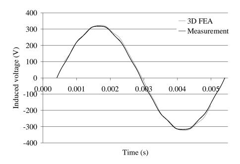
Fig. 4.7. Voltage with the 3D FEA and the measurement. The no-load voltage waveform was measured for the motor equipped with bulky magnets, and it corresponded well with the voltage computed by the 3D FEA.
