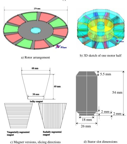
Fig. 4.2. Main dimensions and mechanical arrangements.
