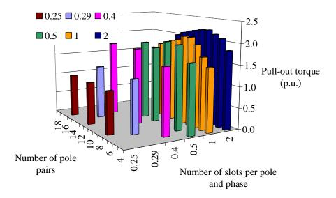
Fig. 3.6. Pull-out torque as a function of p and q for concentrated winding and integral slot winding PM machines.
