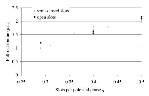
Fig. 3.7. Pull-out torques of some concentrated winding machines with rotor surface magnets (Lindh et al 2009).
