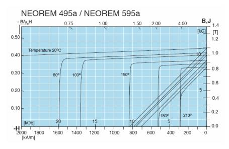
Fig. 1.3. Demagnetization characteristics of NEOREM 495a/NEOREM 595a NdFeB permanent magnet material at different temperatures (Neorem Magnets, 2009).
