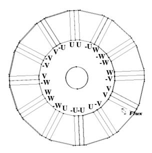
Fig. 4.1. Locations of the stator coil sides in slots
