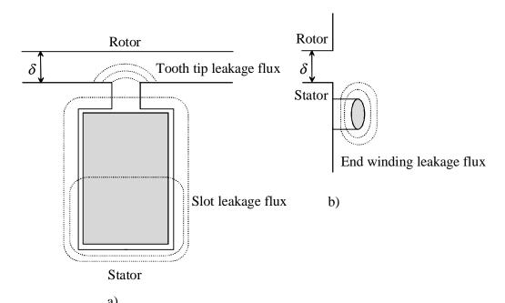
Fig. 2.10. Leakage flux components. a) Slot and tooth tip leakage flux and b) end winding leakage flux.
