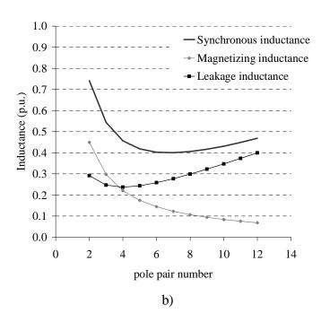
Fig. 3.4. a) Synchronous inductance  $L_{\rm d}$ , magnetizing inductance  $L_{\rm md}$  and leakage inductance  $L_{\rm so}$  of a concentrated winding (q=0.5) machine as a function of pole pair number. b) Corresponding values of integral slot winding (q=2) machines as a function of pole pair number (Jussila et al. 2007)
