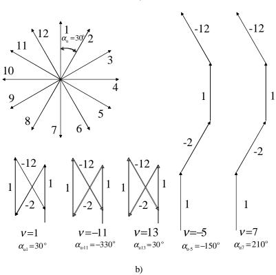
Fig. 1.4. a) Winding arrangement of a 12-10-machine. b) Voltage phasor graph for the fundamental and sum phasors for different harmonics of the 12-10-two-layer winding for phase U located in slots 12-1 and 1-2.
