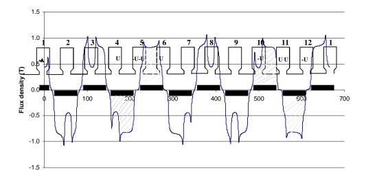
Fig 2.10 Air gap flux density and the permanent magnet positions of a radial flux machine or an axial flux machine at a certain radius. The x-axis co-ordinate is given in mm for the machine observed. Calculating the maximum flux of a pole can be done in such a pole where the magnet and the tooth observed are aligned (in this case between 200 mm and 300 mm).
