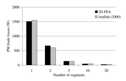
Fig. 2.16. Stator-harmonic-caused PM Joule losses calculated analytically by the Atallah et al. (2000) method and the 2D FEA for a 12-slot-10-pole machine. One magnet is segmented into 20 pieces at maximum.
