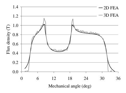
Fig. 2.9. Axial flux motor air gap flux density waveforms: the 2D and 3D analyses along one pole pitch. In 3D, the ripple is caused by the FEA net quality. Bad elements are always present in 3D. Their amount is typically in the range of 4 %. Local mistakes are emphasized but for example the flux integral is usually fairly accurate.
