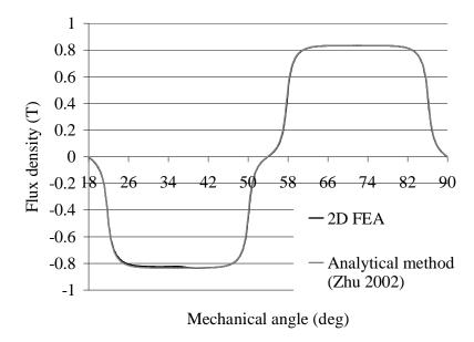
Fig. 2.6. Comparison of the air gap flux densities using the analytical method (Zhu et al. 2002) and 2D FEA. A good match is seen.
