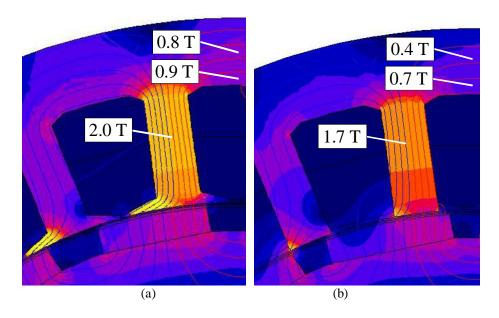
Fig. 1.2. Effect of wide and narrow tooth tips on the flux of otherwise similar machines. The flux paths and flux densities of a 24-slot 16-pole machine a) with semi-closed slots and b) with open slots are shown (Lindh et al. "Concentrated Wound PM Motors with Semiclosed Slots and with Open Slots." *IEEE Energy Conversion* (forthcoming).
