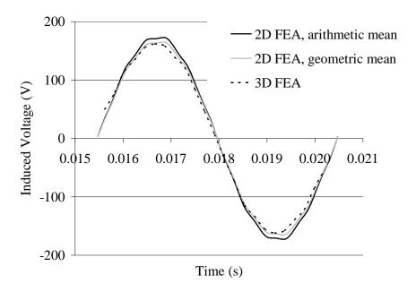
Fig. 2.4. Induced back-emf voltage over one pole pitch with the geometric mean radius (2D FEA using  $l' = l_{\text{Fe}}$ ), the arithmetic mean radius (2D FEA) and the 3D FEA.
