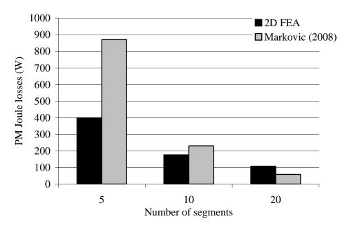
Fig. 2.19. Permeance-harmonic-caused PM Joule losses calculated analytically by the Markovic and Perriard method (2008) and by the 2D FEA for a 12-slot-10-pole machine. One magnet is segmented into 20 pieces at maximum.
