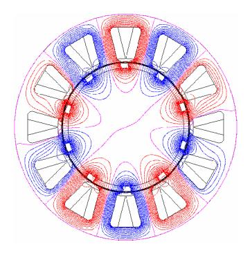
Fig. 2.1. Flux paths of a 12-slot 10-pole radial flux machine. The machine can be divided only into two magnetically symmetric parts. It means that there are five different flux paths in different poles.
