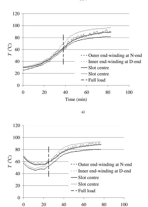
Fig. 4.10. Temperatures at rated loads. a) Radially segmented and b) tangentially segmented magnets at 2400 min<sup>-1</sup>.
