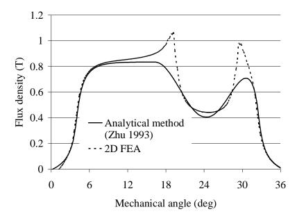
Fig. 2.8. Slotting effect applying the Zhu and Howe method (1993) and the 2D FEA.
