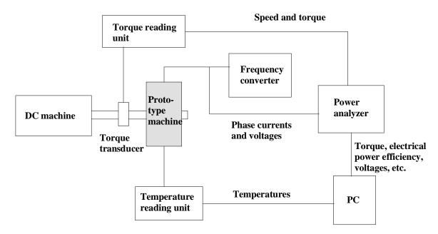
Fig. 4.6. Load test arrangement for the concentrated winding axial flux PM. The measured prototype motor was supplied by a frequency converter. The torque and the rotating speed were measured with a Vibrometer torque transducer. The electric power was measured with a Yogokawa PZ4000 power analyzer equipped with three current transformers. Four thermoelements were mounted in the stator windings and two in both stators for temperature analyses. A Fluke Hydra 2620A measured the temperatures.
