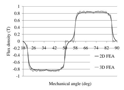
Fig. 2.7. Comparison of the air gap flux densities by the 2D and 3D FEA. The coarse form of the 3D result is a consequence of sparse elements.
