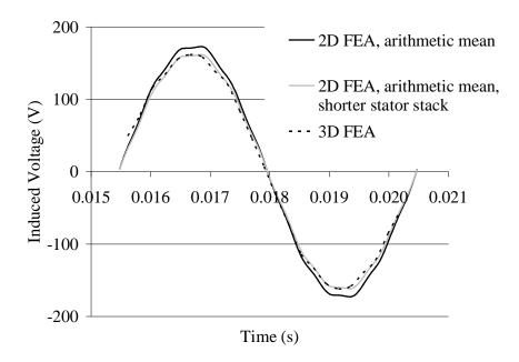
Fig. 2.5. Induced back-emf voltage over one pole pitch with the arithmetic mean radius (2D FEA using  $l' = l_{Fe}$ ), the arithmetic mean radius (2D FEA using  $l' = l_{Fe} - 2\delta$ ) and the 3D FEA.
