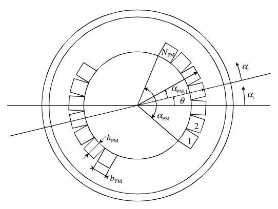
Fig. 2.15. Cross-section of the two-pole PM machine (Polinder and Hoeijmakers 1999).
