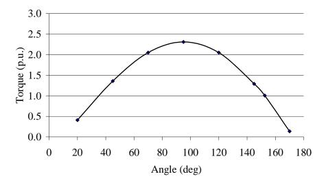
Fig. 4.12. Torque curve as a function of load angle for the segmented (20 pieces) magnet machine.
