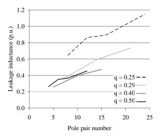
Fig. 3.2. Leakage inductances of concentrated winding machines with numbers of slots per pole and phase q = 0.25, 0.29, 0.4 and 0.5 (Jussila et al. 2007).
