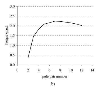
Fig. 3.5. a) Maximum pull-out torque of a concentrated winding (q = 0.5) machine as a function of pole pair number. b) Corresponding value of an integral slot winding (q = 2) machine as a function of pole pair number (Jussila et al. 2007).
