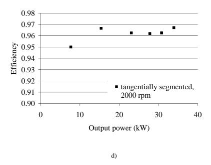
Fig. 4.9. Measured efficiencies with radially and tangentially segmented magnets at 2400 and  $2000 \, \text{min}^{-1}$ .
