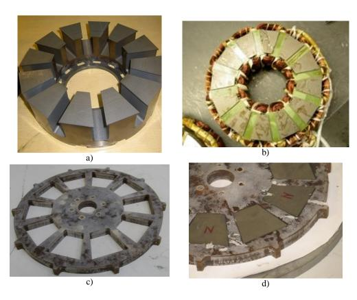
Fig. 4.4. a) Stator lamination stack, b) one stator equipped with windings, c) rotor frame, d) rotor with magnets assembled
