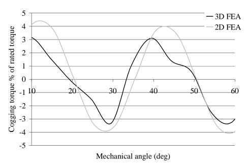
Fig. 4.13. Peak-to-peak values of the cogging torque in (%) of the rated torque with the 2D and 3D FEA.
