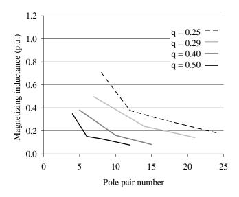
Fig. 3.1. Per unit magnetizing inductances of concentrated winding machines with numbers of slots per pole and phase q = 0.25, 0.29, 0.4 and 0.5 (Jussila et al. 2007).
