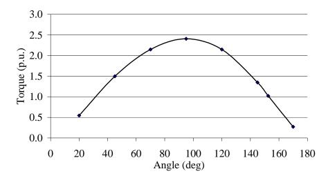
Fig. 4.11. Torque curve as a function of load angle for the bulk magnet machine.
