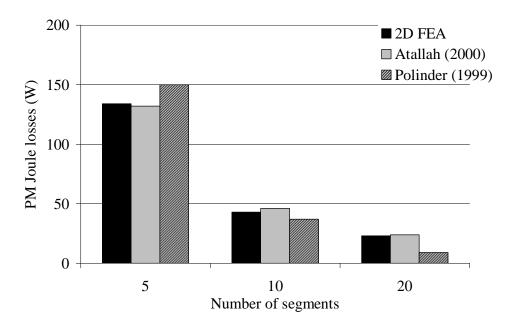
Fig. 2.17. Same results as in the previous figure calculated analytically by the methods by Atallah et al. (2000) and Polinder and Hoeijmakers (1999) and the 2D FEA for a 12-slot-10-pole machine. One magnet is segmented into 20 pieces at maximum.
