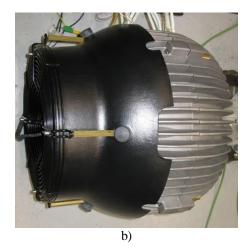
Fig. 4.5. Motor without a fan and with an externally operated fan.
