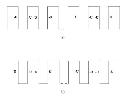
Fig. 2.12. a) All coils in one phase (U) for a concentrated winding q=0.4 and b) All coils in one phase (U) for an integral slot winding q=2,  $W/\tau_p=5/6$ .
