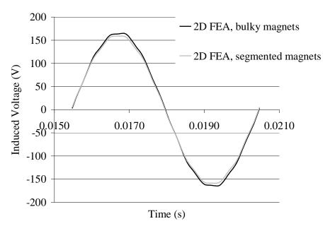
Fig. 4.8. Effect of segmentation. The voltage drop is proportional to the change in volume of the magnet mass when segmented magnets (20) are used. Half of the axial flux machine (one stator) is modelled to the radial flux machine.
