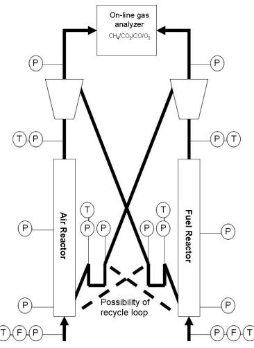
Figure 34. Locations for measurements at reactor design, P pressure, T temperature, F flowmeter
