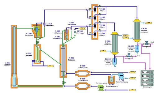
**Figure 13.** Schematic diagram of a  $50 \text{kW}_{th}$  chemical-looping combustion system. (Ryu et al. 2004)
