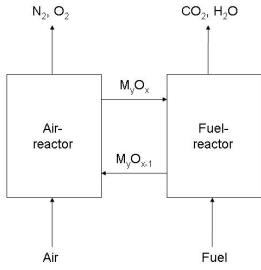
Figure 1. Basic concept of CLC-process and oxygen carrier circulation (Johansson 2007)
