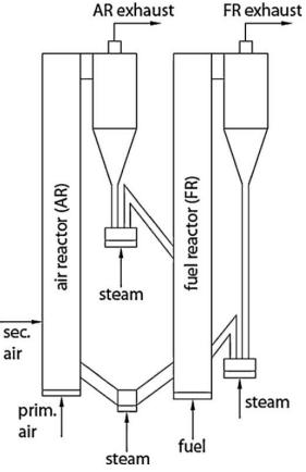
**Figure 15.** DCFB reactor system set-up. Both AR and FR are designed as circulating fluidized beds. Kolbitsch et al. (2010)
