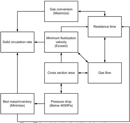
Figure 27. Interrelationship of variables during sizing
