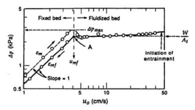
**Figure 2.** Pressure drop versus gas velocity for a bed of uniformly sized sand particles (Kunii & Levenspiel 1977)
