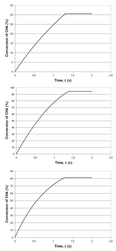
Figure 28. Conversion of fuel at fuel reactor, Fe-, Cu- and Ni-based oxygen carrier, particle diameter  $200 \mu m$
