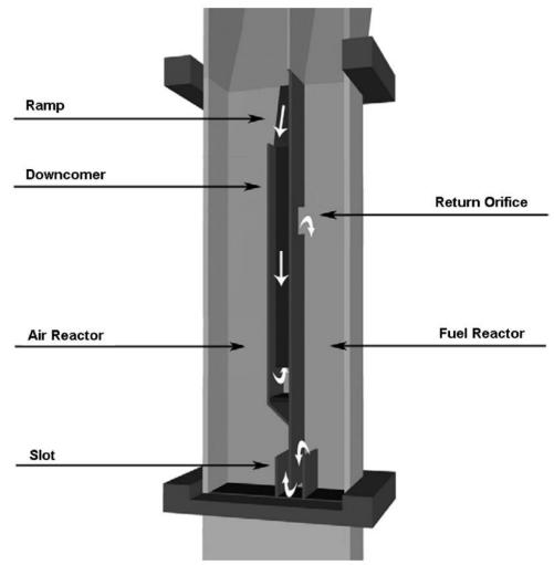
**Figure 8.** Schematic description of the improved reactor for oxygen carrier tests. (Rydén et al. 2008)
