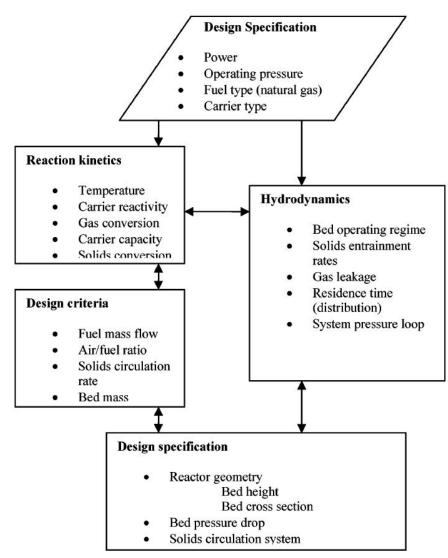
Figure 12. Design procedure of a chemical-looping combustor. (Kronberger et al. 2004)
