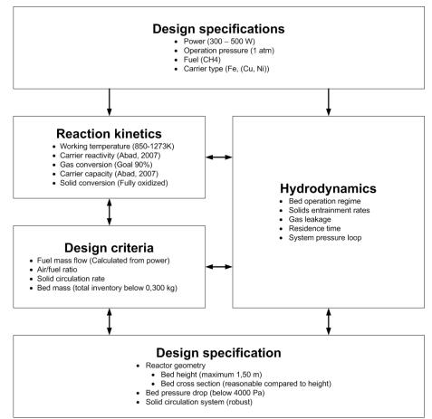
Figure 26. Design procedure with fixed properties and initial conditions
