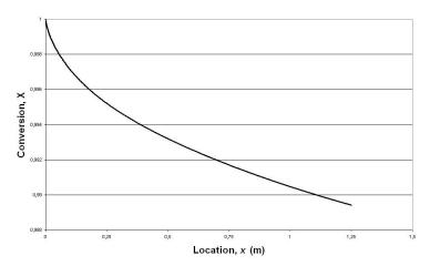
Figure 25. Conversion state of oxygen carrier at fuel reactor
