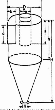
Figure 31. Cyclone shape and dimensions
