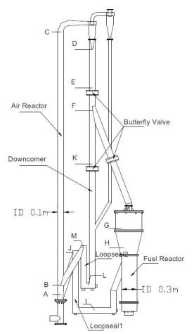
Figure 6. Reactor design with recycle loops. (Xu et al. 2009)
