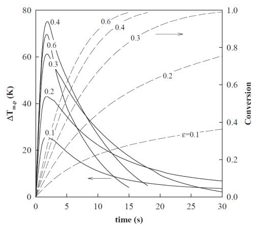
**Figure 3.** Effect of porosity on the maximum temperature increase inside of the particle during the Ni oxidation. (Garcia-Labiano et al. 2005)
