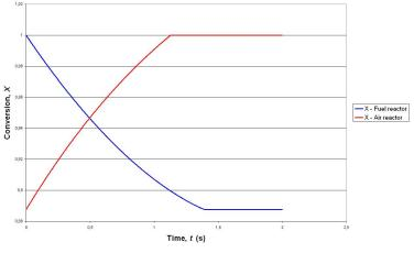
Figure 30. Conversion of Cu-based oxygen carrier
