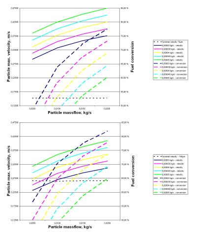
Figure 29. Parameter run of Fe-based oxygen carrier at fuel reactor with different gas mass flow, particle diameter  $75 \mu m$  and  $100 \mu m$
