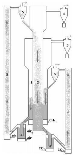
**Figure 10.** Schematic diagram of CFB reactor for CLC. (1) Reduction zone, annular column, 55 mm i.d., 0.9 m height; (2) oxidation zone, inner column, 23 mm i.d., 1.5 m height; (3) riser, 17 mm i.d., 2.1 m height for oxidizer, 1.15 m height for reducer; (4) loop-seal, 23 mm i.d., seal-pot type; and (5) cyclone.
