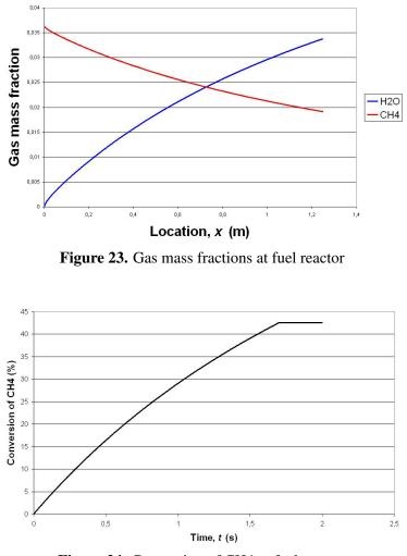
Figure 24. Conversion of CH4 at fuel reactor
