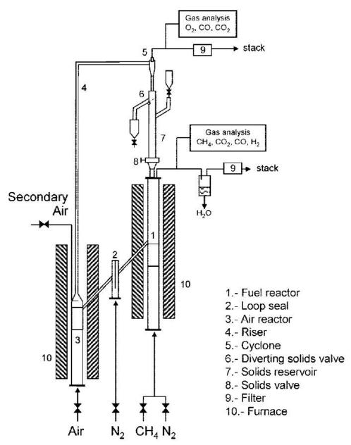
Figure 9. Schematic description of 500W reactor. (Adánez et al. 2009)
