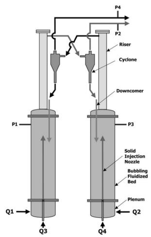
**Figure 18.** Schematic of a two bubbling bed interconnected circulating fluidized bed system. (Ryu et al. 2008)
