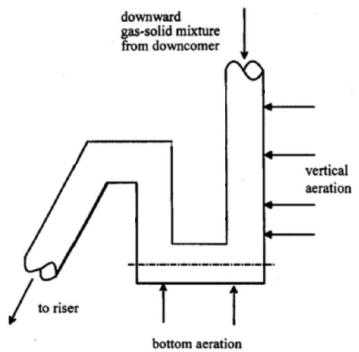
Figure 32. Schematic diagram of loop-seal (Kim et al. 1999)
