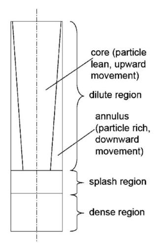
**Figure 14.** Typical structure of fluid dynamic description of fast fluidized bed reactors Kolbitsch, Pröll & Hofbauer (2009)
