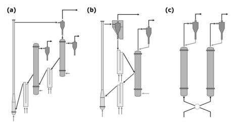
**Figure 17.** Schematic of conventional two interconnected circulating fluidized bed system. (Ryu et al. 2008)
