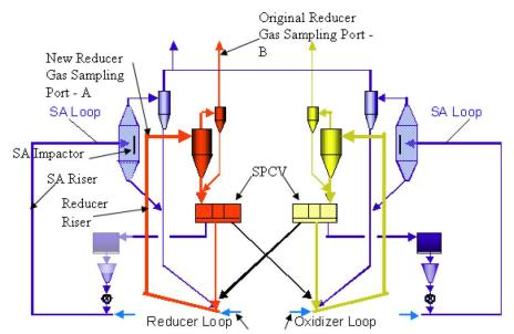
Figure 16. Schematics of reactor by Alstom Power Inc. (Abdulally et al. 2010)
