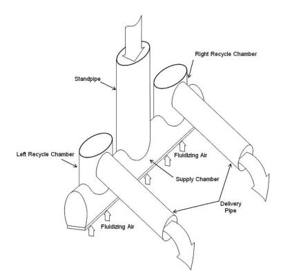
**Figure 33.** Loop-seal of a large commercial CFB boiler with a twin recycle chamber (Basu et al. 2009)
