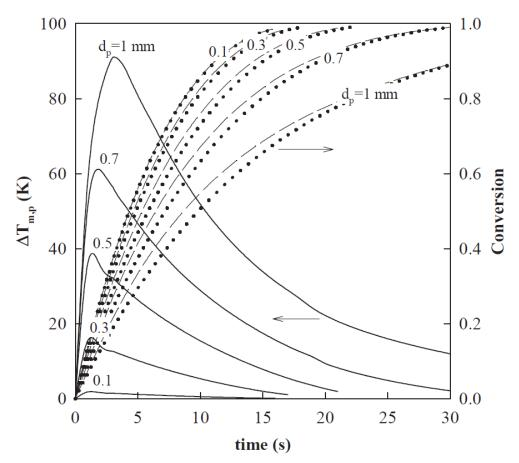
**Figure 4.** Effect of particle size on the solid conversion and the maximum temperature increase inside of the particle for the Ni oxidation reaction (dotted line = isothermal particles). (Garcìa-Labiano et al. 2005)
