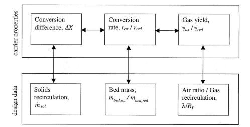
**Figure 11.** The basic relations between carrier reactivity and design input data. (Lyngfelt et al. 2001)
