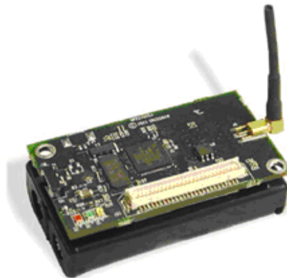
Figure 9. Actual MICAZ Hardware [32]
