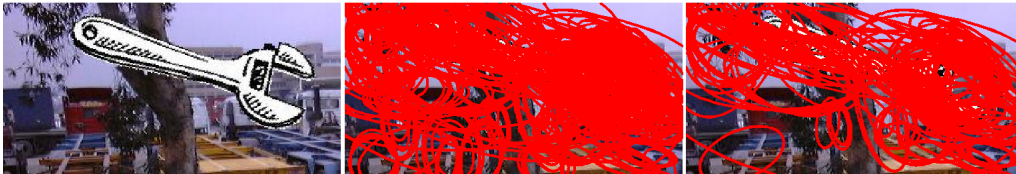
Figure 3.3: Local feature filtering sample outputs using Randomised Caltech-101: Left: Original image (wrench); Middle: All the extracted Hessian-Affine local features; Right: Local features after filtering uncommon features out.
