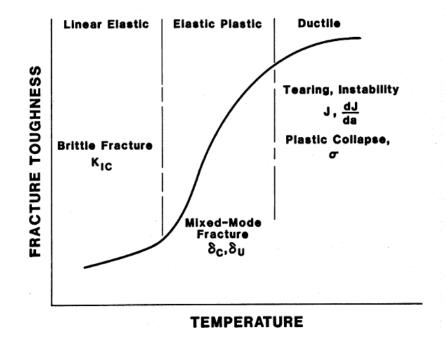
**Figure 1.0:** The ductile-brittle transition of steel showing brittle (linear elastic), elastic-plastic and ductile (fully plastic) regions [3]
