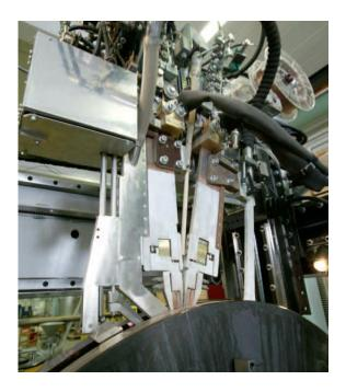
Figure 2.3.3: Narrow Gap Welding head [26]
