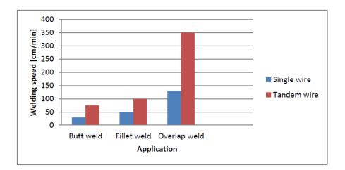
**Figure 2.3.13:** Comparison of welding speeds for the single wire and tandem wire applications [48]
