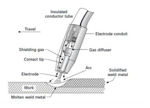
**Figure 2.3.8:** Schematic representation of MIG/MAG process (Longitudinal-Section View) [49]
