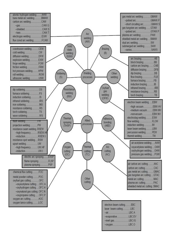
**Figure 1.1.1:** Master Chart of Welding and Allied Processes Source: Welding Inspection Technology, American Welding Society (AWS) [5].
