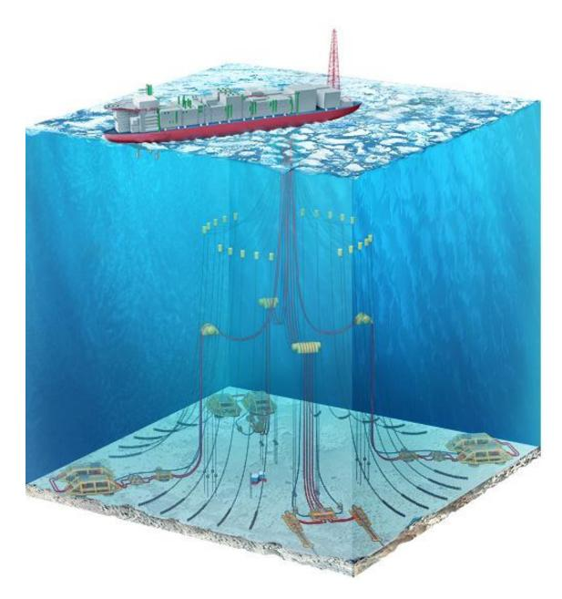
Figure 4.3: The offshore facilites for Shtokman project [63]
