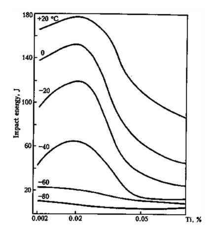
**Figure 3.2.2:** Influence of titanium content in weld metal on impact energy at different temperature [61]
