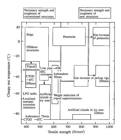
**Figure 2.1:** Changes in strength and toughness required in the energy development field [17]
