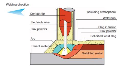
Figure 2.3.14: Schematic representation of SAW process [51]
