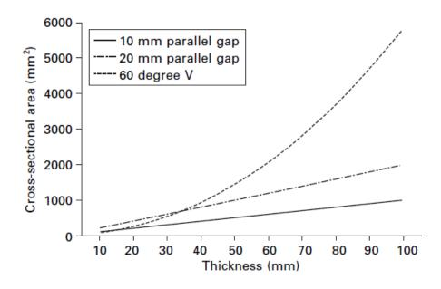
**Figure 2.3.2:** The principle of narrow-gap welding: The effects of joint preparation on weld cross-sectional area [24].
