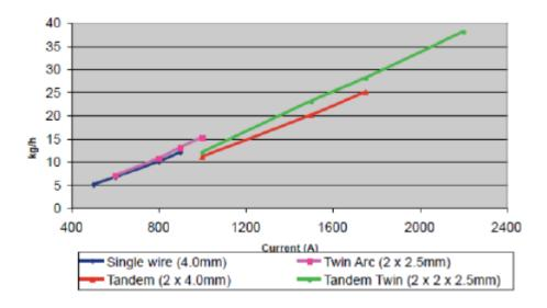
Figure 2.3.19: SAW process variations and their deposition rates [53]
