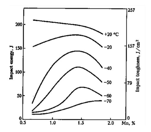
**Figure 3.2.1:** Influence of manganese content on impact energy and impact toughness of weld metal at different temperature [58]
