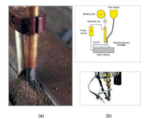
Figure 2.3.16: Core wire variation (a) and Single wire variation (b) [53]
