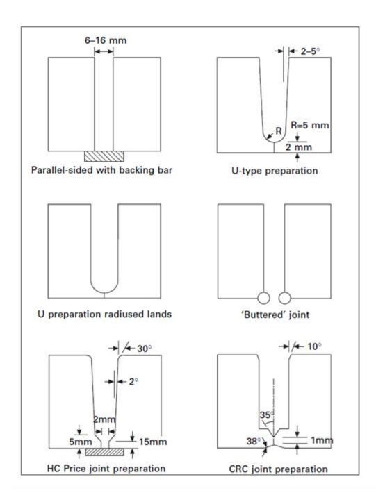
Figure 2.3.1: Typical narrow-joint Preparation. [25]
