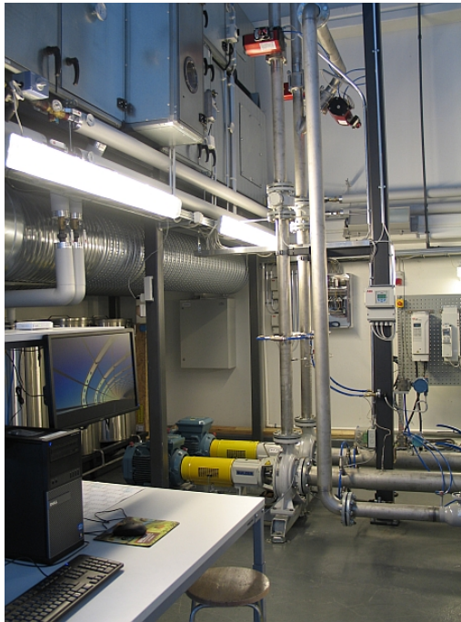
Fig. 4.1 The measurement system used in laboratory evaluation. The core components are the measurement device (PC with installed LabVIEW™), a frequency converter, an induction motor and a centrifugal pump.
