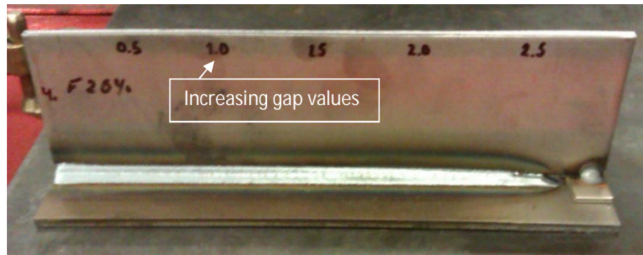
Figure 50. Increasing gap values sample using WiseFusion™, 20% short circuit.
