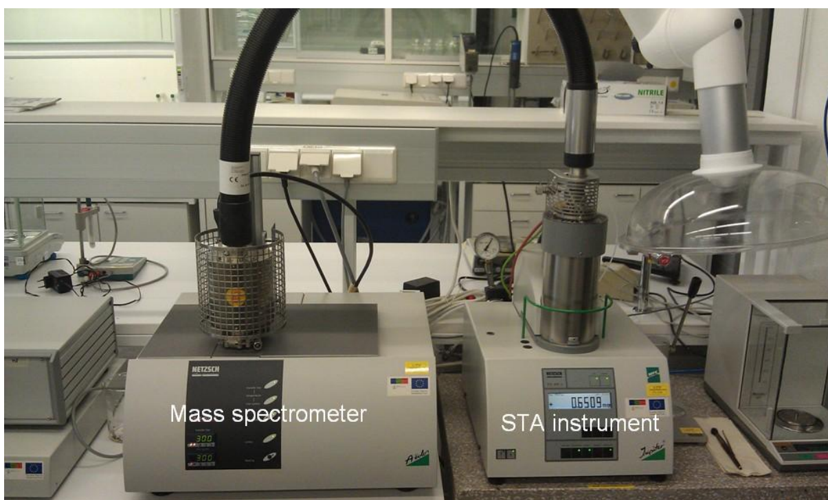
Figure 5.2. Laboratory installation for thermal balance tests.
