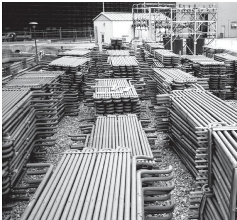
Figure 2.7. Auxiliary superheater components [5].
