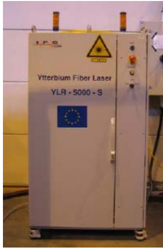
Figure 11. The YLR-5000-S multi-mode fiber laser.
