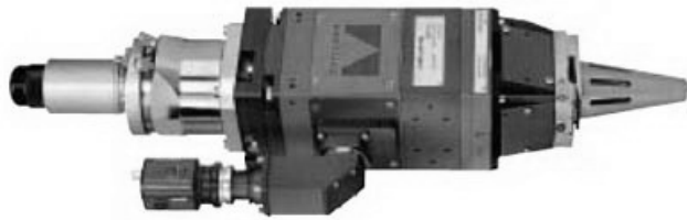
Figure 12. Precitec YW50 laser head. 73
