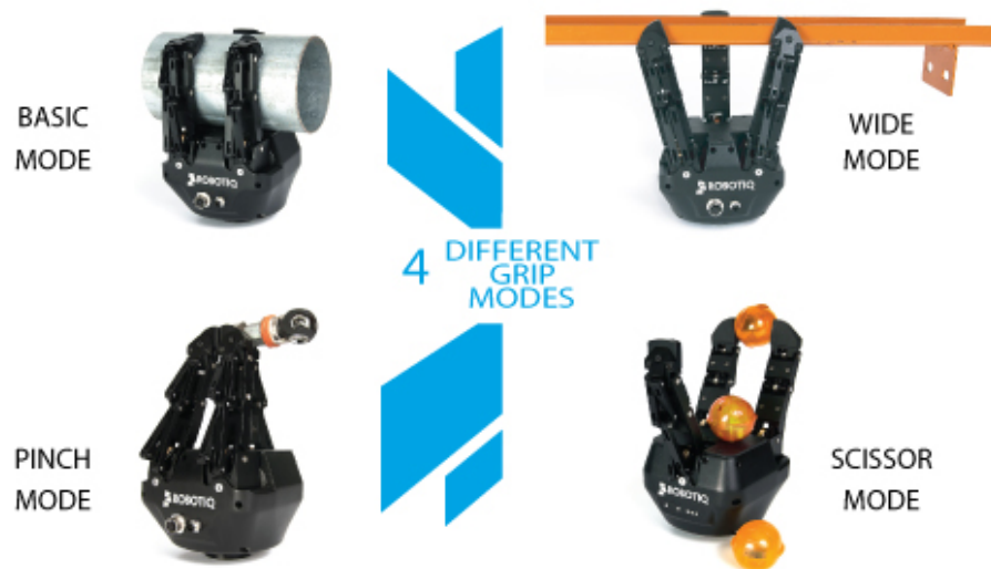
Figure 2. The four build-in modes of the gripper[11].
