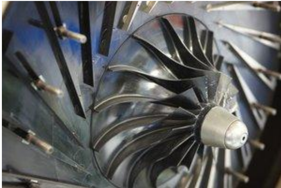
Figure 13. The impeller and diffuser of RADIVER compressor (22)
