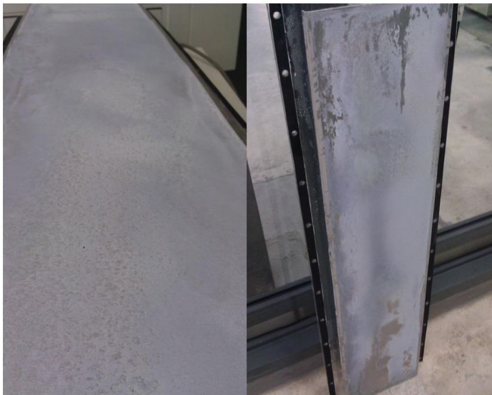
Figure 17. The rear plate electrode with catalyst before (left) and after (right) the experiments.
