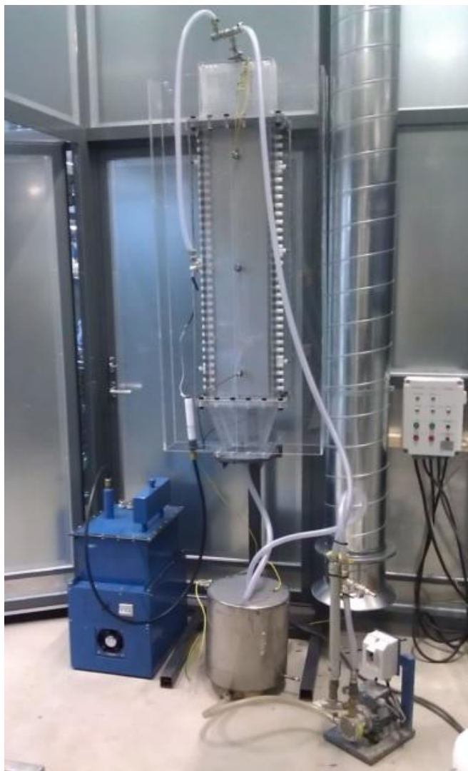
Figure 3. The experimental setup: pulse generator (left), PCD reactor (middle above), solution tank (middle below) and pumping unit with flow control and sampling valve (bottom right).
