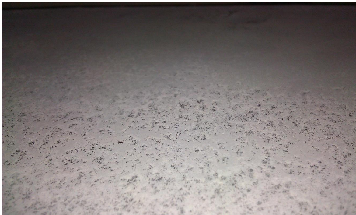
Figure 12. A plate electrode surface with titanium dioxide coating.
