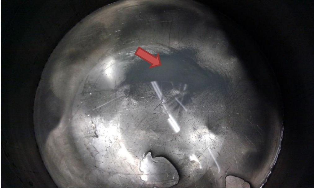
Figure 15. Loose titanium dioxide particles in the tank bottom after fifth catalytic treatment of oxalic acid (833 pps).
