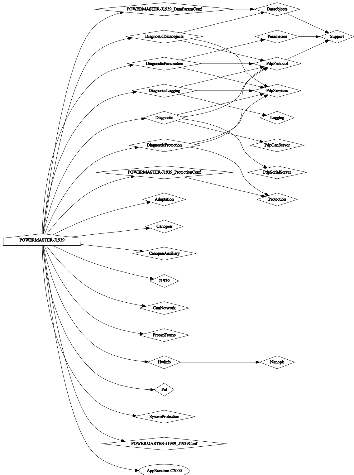
Figure 20. Component dependency graph of the PowerMASTER J1939 communication variant using the dependency output function of the generator tool.
