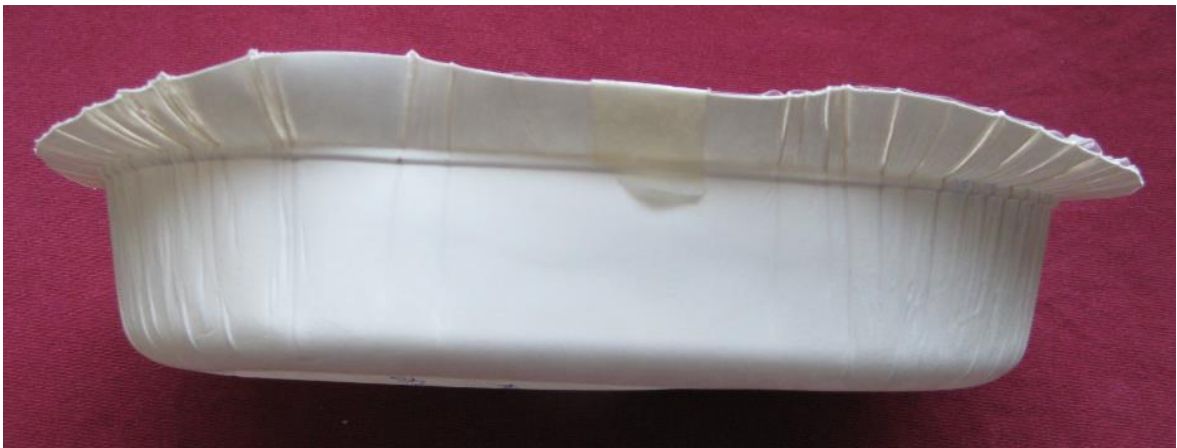
Figure 29. Deformed paperboard due to high temperature (160 0 C).
