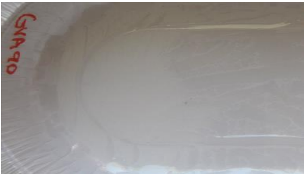
Figure 28. Air bubble formation during pressing of MULTIFOL GVA 90 coated paperboard.
