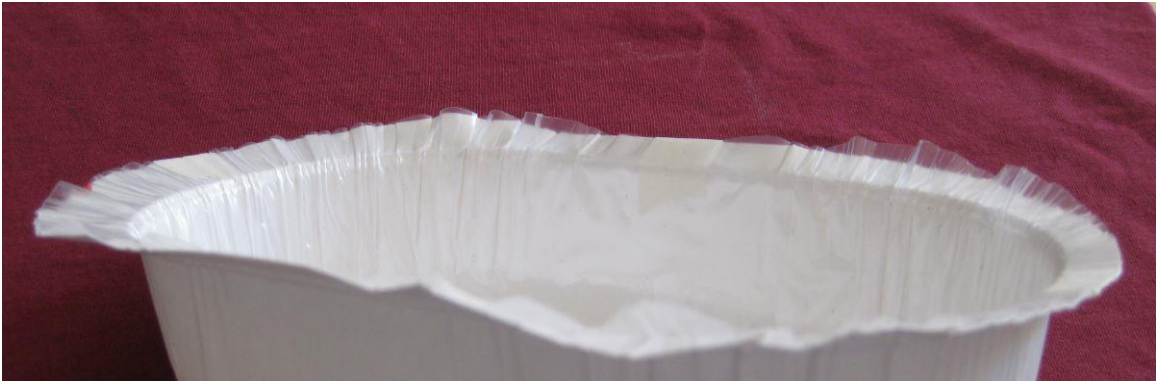
Figure 30. Defects at the edge of tray when coating Performa Natura with MULTIFOL SV 100.
