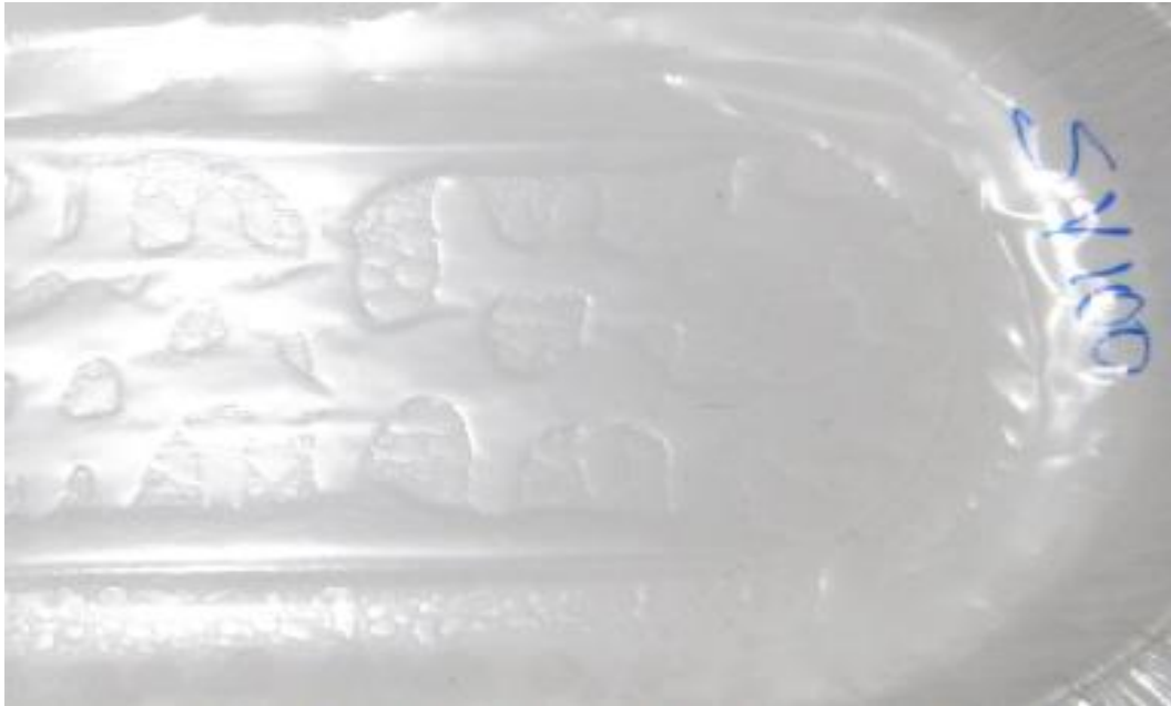
Figure 27. Air Bubble formation during pressing of MULTIFOL SV 100 coated paperboard.
