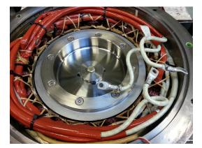
Fig. 3. A photograph of the inside of the 18/16 machine.
