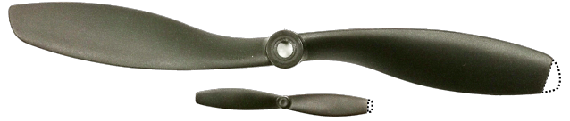
Fig. 3. The damaged propellers used in the experiments, with the removed propeller sections indicated by dashed outlines, on the right-hand side. The damage to the small propeller is approximately 5mg, and that to the large propeller is approximately 40mg.
