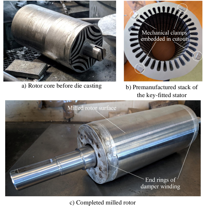
Fig. 16. Motor parts of the 1.5 kW DOLSynRM during manufacturing.
