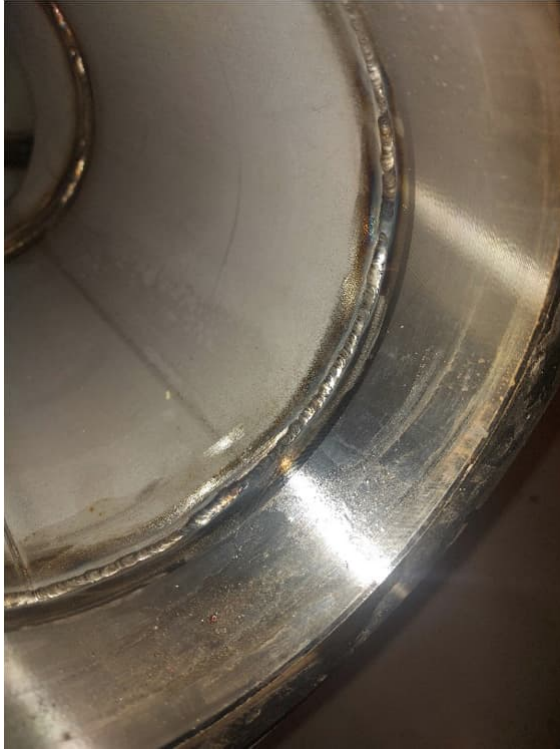
Figure 16 In the welds, a high root dome, bluing, and a sharp junction were noticed (Case Company, 2022).
