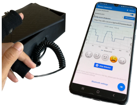
Figure 40: ED used during usability testing: EDA sensor (Left) and adapted version of a mobile app (Right), Mamani 2021 (ibid.)
