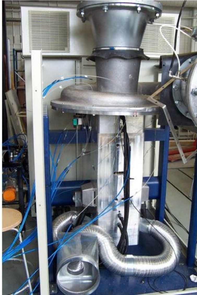
Figure 29. Centrifugal compressor test station (Turunen-Saaresti Teemu 2004, 61)
